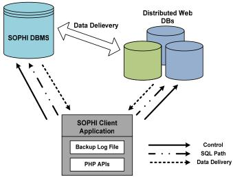
Fig 3.13. WANDA data backup system configuration
